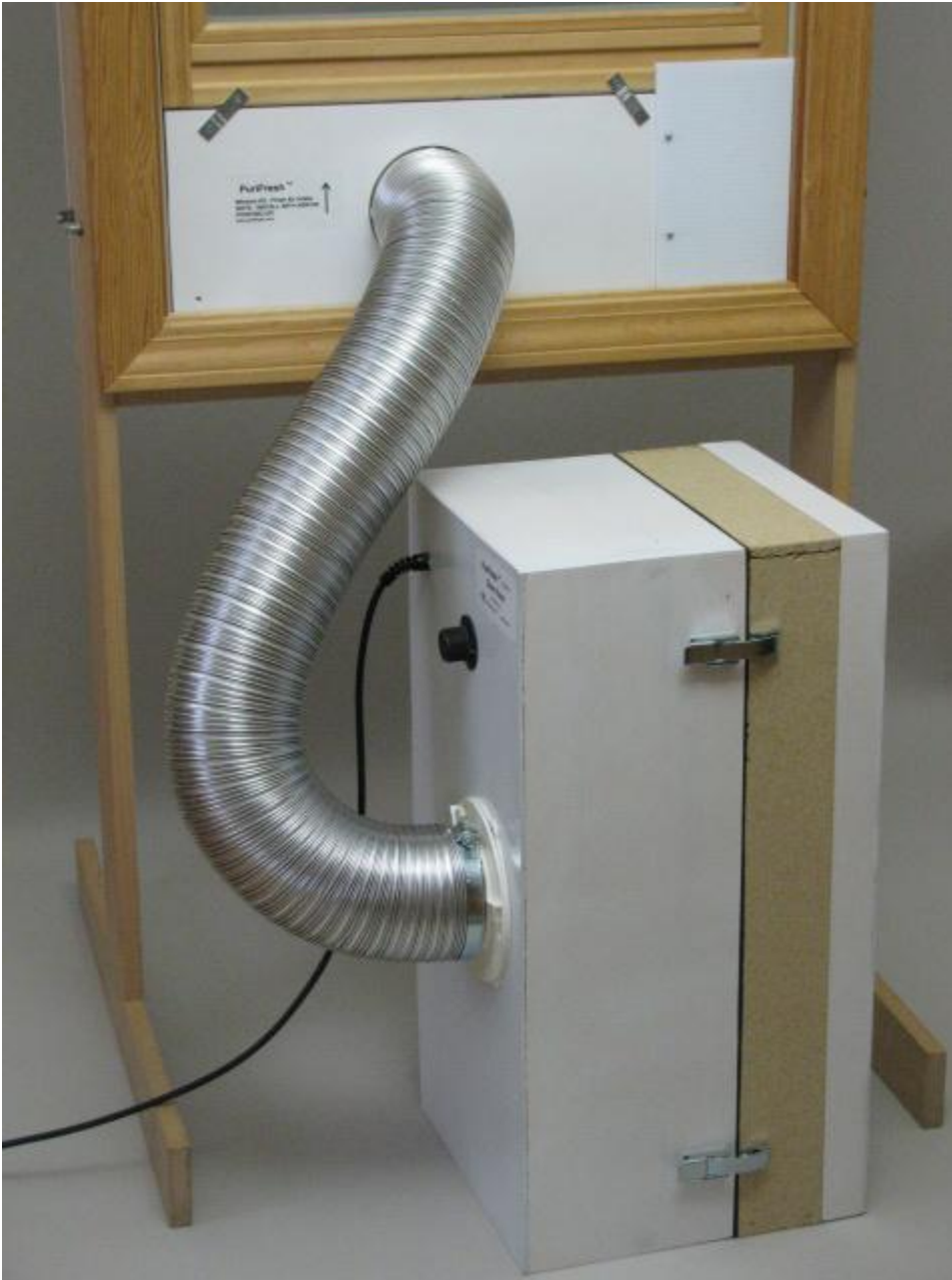
Figure 7: Connect the inlet of the PuriFresh® Clean Room to the Fresh Air Intake of the Window Kit with the flexible 5 inch duct.
